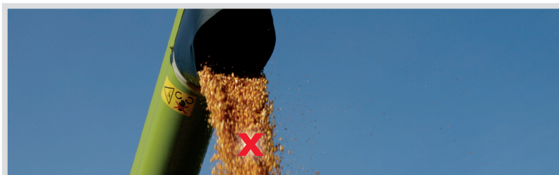
Figure 11. Sampling of grains from the moving stream of a loading spout. The red x represents the spot where the sample should be collected. Collect as many samples as necessary, changing the position of the cup or scoop each time.
