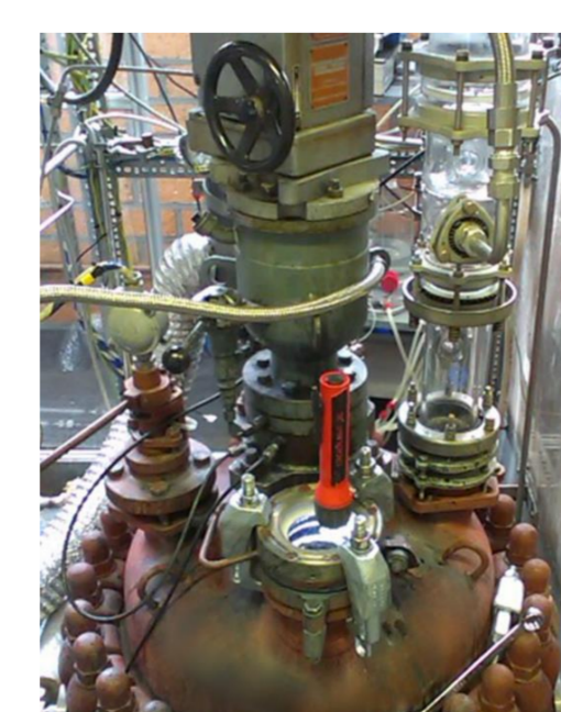
Figure 1. Production of 10-HSA on kilogram scale in the 200 L Reactor Mini Plant
